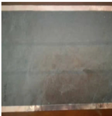
Fig. 9 – Be installed metal copper foil strip as electrical current carrier.
