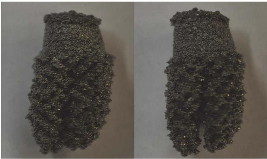
Two bio-adaptable dental implants with porous rootform built by EBM. 18
